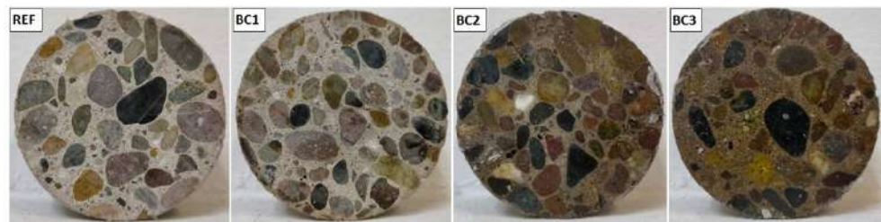
Figure 5. Appearance of the uncoated concrete specimens (REF) and those coated with PPT (BC1, BC2, and BC3).
